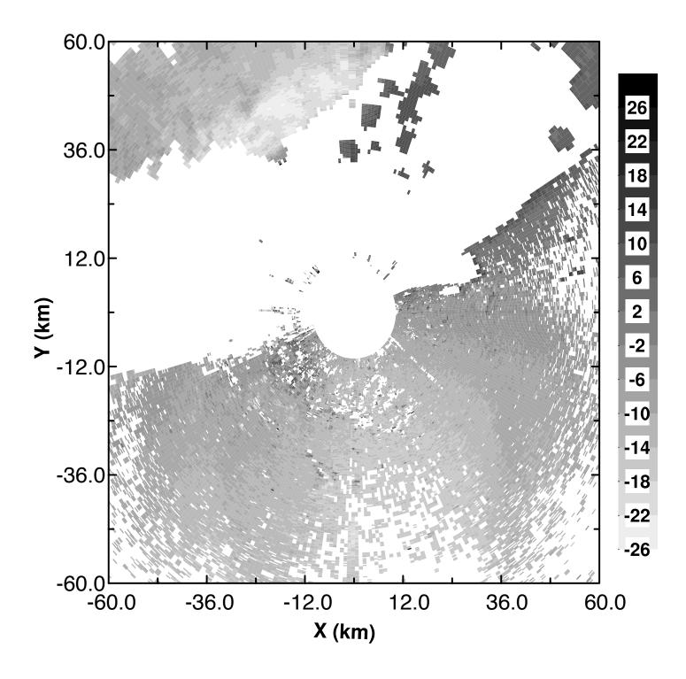
Fig. 6. Dealiased radial velocities on the conical surface of 0.5 degree elevation angle over the area of 120×120 km<sup>2</sup> centered at the radar. The raw radial velocity data were collected by the KTLX radar 0040 UTC on 16 June 2002 for a surface cold front over the area of Oklahoma state.
