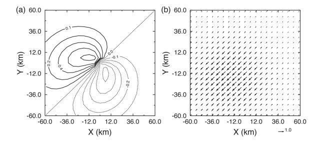
Fig. 1. Cross-correlation function (a), and masked vector velocity field composed of the auto-correlation function and cross-correlation function (b). The two correlation functions are given by (4.2a) and (4.2b) with  $\mathbf{x}_1 = (x_1, y_1) = (-15, -15)$  km and L = 30 km. In panel (a), contours are plotted every 0.1 with solid for non-negative and dotted for negative values.
