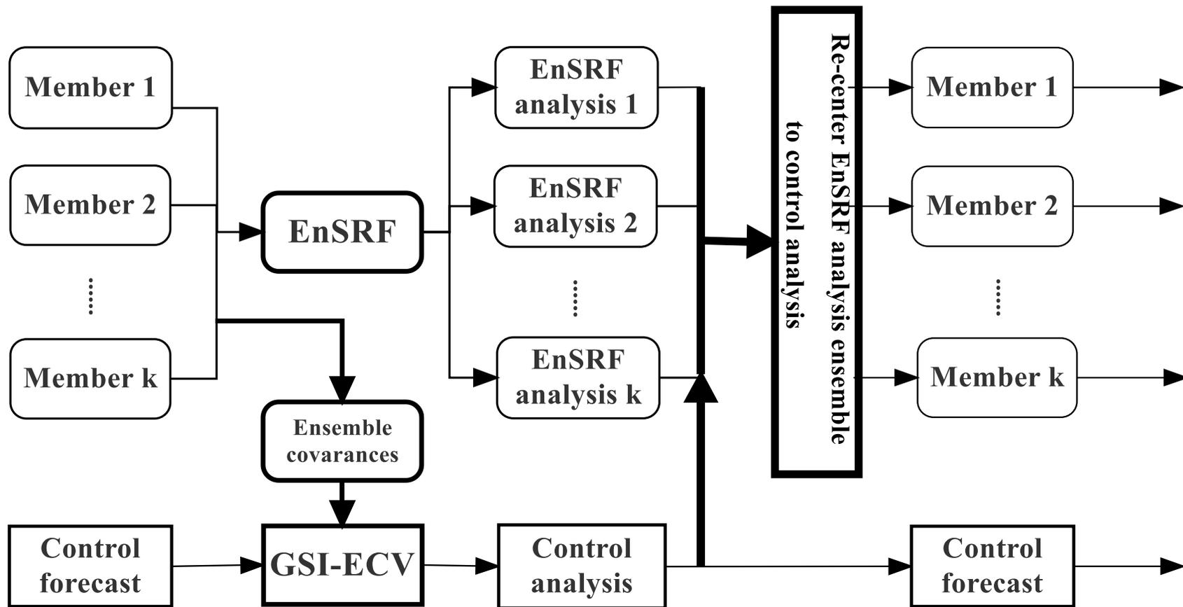
Flowchart of a full EnSRF-En3DVar hybrid data assimilation cycle, with one-way or two-way coupling between the EnSRF (upper portion) and En3DVar hybrid control analysis (lower portion denoted En3DVar). The thick upward pointing arrow indicates the feedback of the En3DVar hybrid analysis to the EnSRF in the two-way coupling procedure, when the En3DVar hybrid control analysis is used to replace the ensemble mean of the EnSRF analyses.
