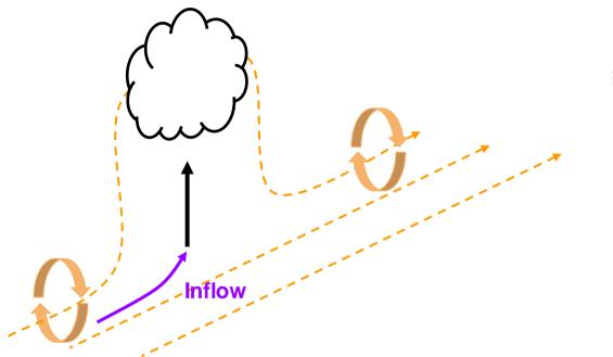
Updraft draws **streamwise** vorticity into the vertical (tilting)
