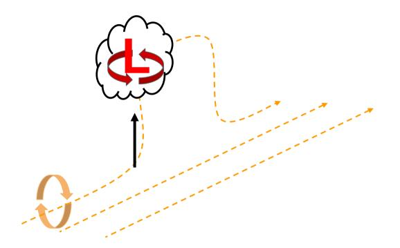
Low pressure perturbation is induced in the vorticity center, which is centered on initial updraft!
