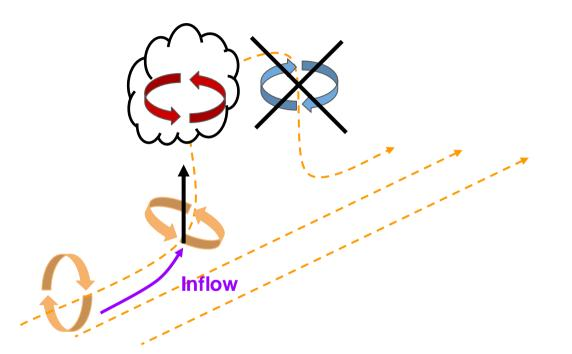
Updraft draws **streamwise** vorticity into the vertical (tilting)
