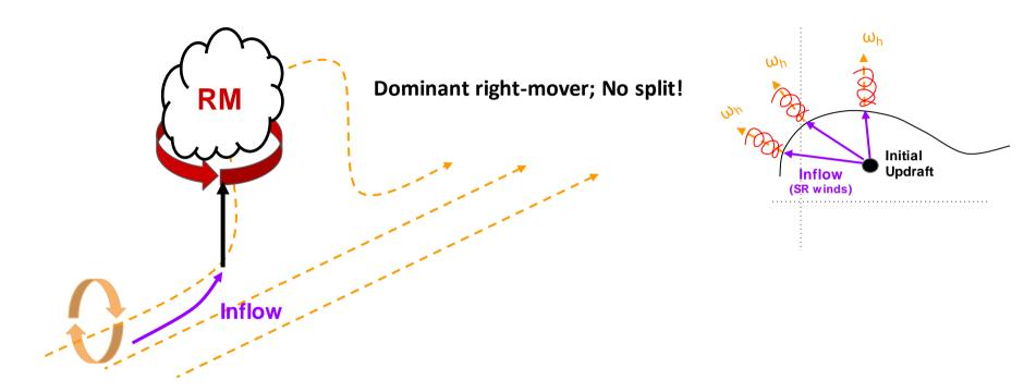
Initial updraft was correlated with the cyclonic vorticity from the start – streamwise vorticity ingestion!
