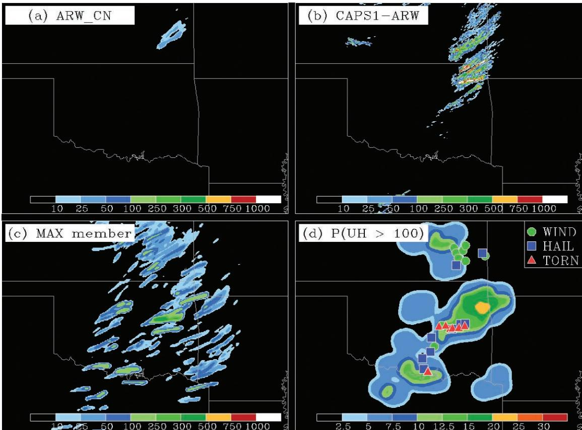
**FIG. 5.** HMF updraft helicity ( $\text{m}^2 \text{s}^{-2}$ ) from 25-h forecasts initialized 0000 UTC 10 May 2010 from (a) the ARW control member of the SSEF system and (b) the CAPS run with 1-km grid spacing. (c) Maximum HMF updraft helicity from any SSEF member. (d) Neighborhood probabilities for updraft helicity greater than  $100 \text{ m}^2 \text{s}^{-2}$ , and storm reports that occurred between 0000 and 0100 UTC 11 May (legend in top right).
