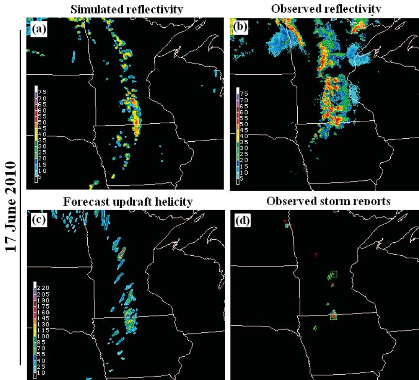
**FIG. 10.** (a) Simulated 1-km AGL reflectivity (dBZ) at forecast hour 5 (valid 2300 UTC) from the 1800 UTC 17 Jun 2010 initialized HRRR, and (b) corresponding observed base reflectivity (dBZ). (c) As in (a), but for forecast hourly maximum updraft helicity ( $\text{m}^2\text{s}^{-2}$ ), and (d) observed storm reports between 2200 and 2300 UTC 17 Jun 2010 (green “A”s indicate hail, blue “W”s and “G”s indicate wind, and red “T”s indicate tornadoes).
