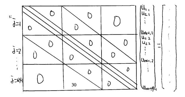
This system cannot be solved as efficiently as the tridiagonal system from 1-D problem. Similar system arises from the discretization of elliptic equation  $\nabla^2 u = F$ . We will discuss methods for solving it at a later time.
