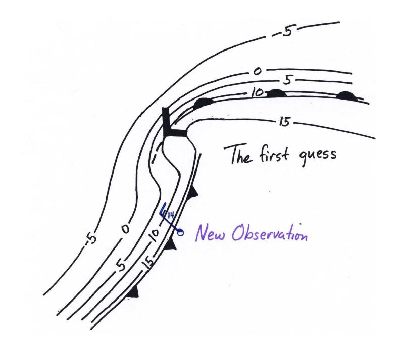
New observation is inconsistent with first guess 3D-Var produces an unappealing analysis, bowing the front out just in the region of the observation.
