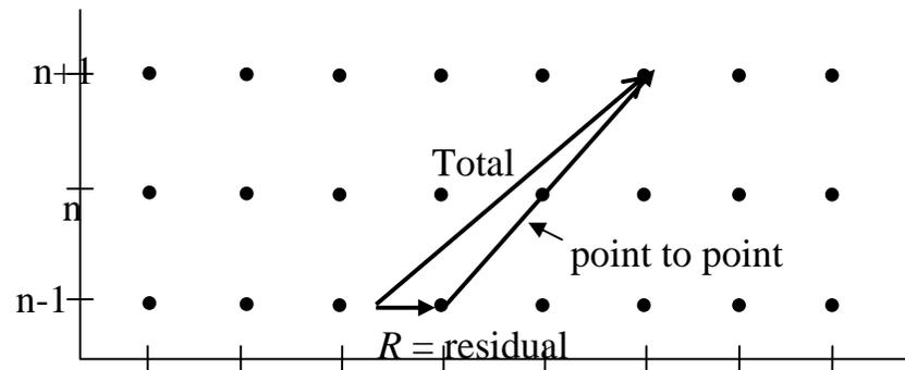
The mesh-point to mesh-point vector is simple replacement since the values at grid points are always known. The residual  $R$  is handled using an Eulerian approach, which requires that  $|u\Delta t/\Delta x| \leq 1$ .
