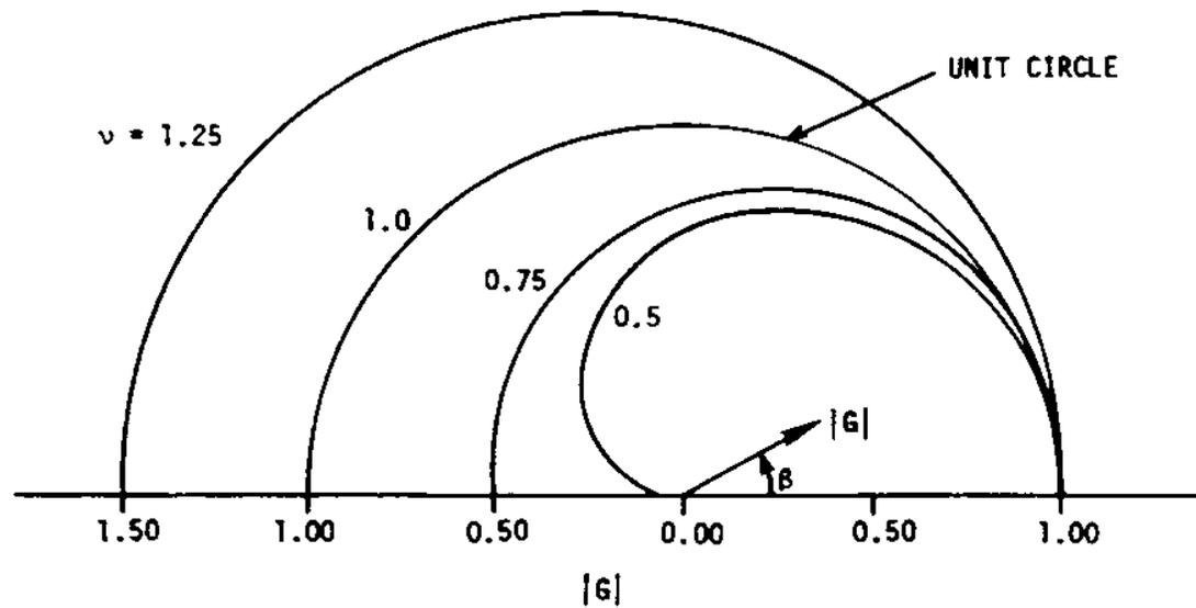
**Figure 4.2** Amplification factor modulus for upstream differencing scheme.
