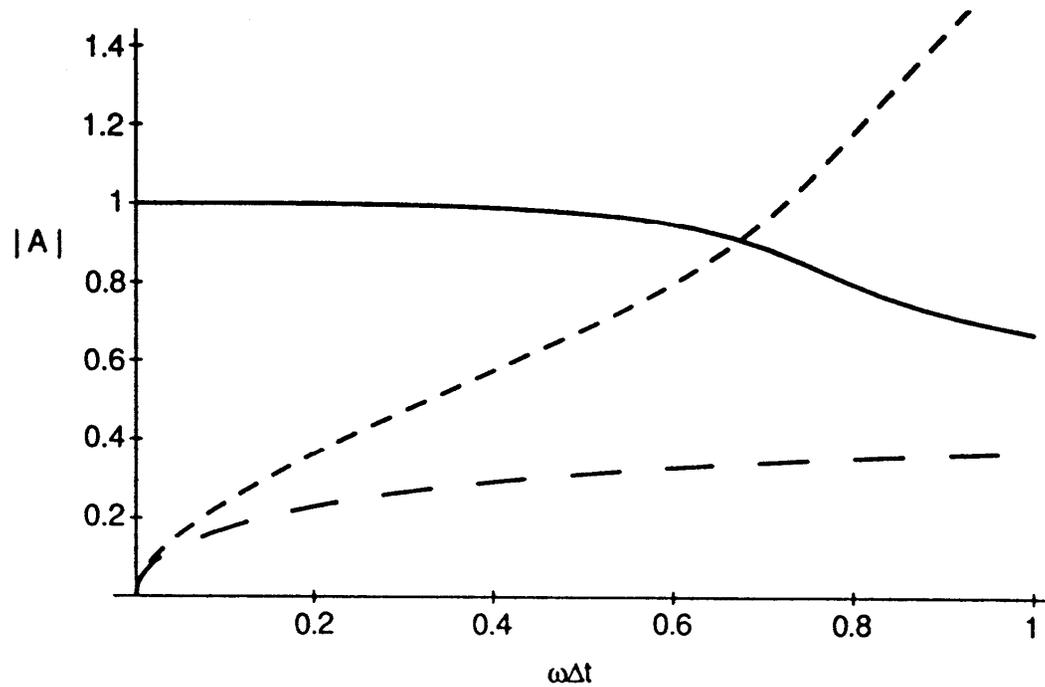
FIG. 1. Magnitude of the amplification factor for the third-order Adams-Bashforth scheme plotted as a function of  $\omega\Delta t$ . Solid line is the physical mode; dashed curves are the two computational modes.
