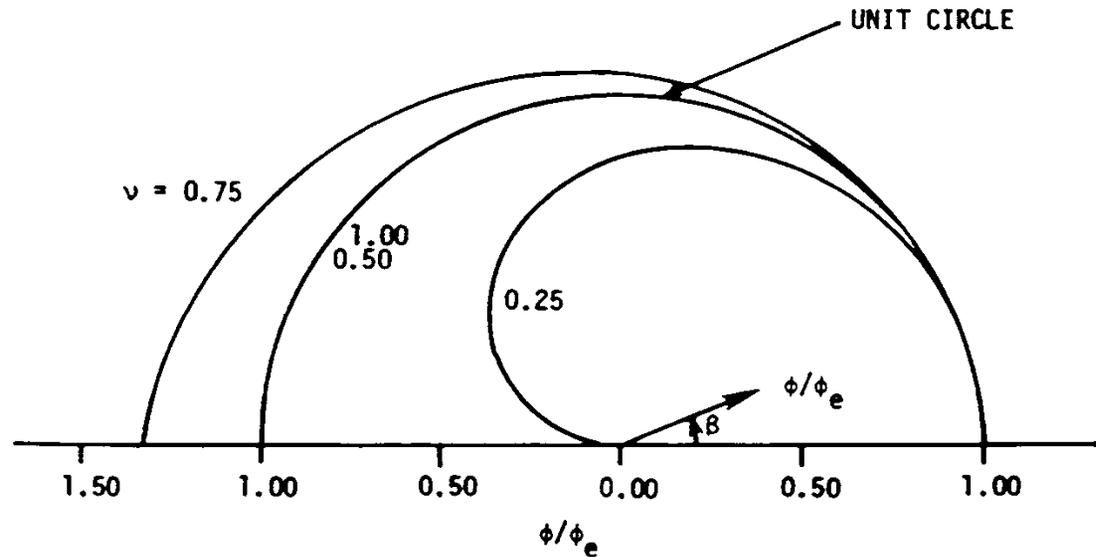
Figure 4.3 Relative phase error of upstream differencing scheme.
