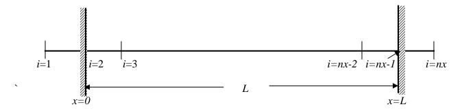
In the discrete form, the boundary conditions are: u(1) = u(nx-2) and u(nx) = u(3). When these conditions are used, u(2) = u(nx-1)) should be automatically satisfied (note a typo with the previous version of this formula). For actual implementation, you integrate the finite difference equation forward in time for i = 2 to nx-1, and set boundary conditions at i = 1 and nx.
